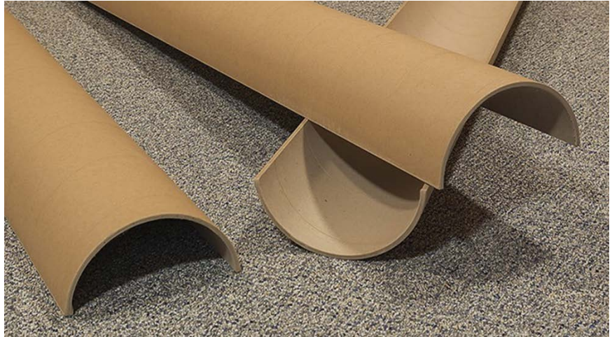
Figure 2 The inexpensive cardboard concrete forms, cut in half, that have proven to serve an extremely useful purpose in upgrading the acoustical signature of large spaces.
